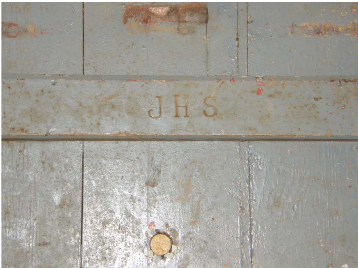
The BPB Co practice was to stamp the yard number under the floor inspection panels on the larger military boats and “Makaira’s” panel has JHS stamped underneath, showing the boat was in build for J.H. Storey. (Photo Jon Blair)
